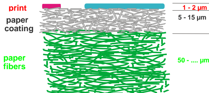
Fig. 1 Proportions of thicknesses in a coated paper
