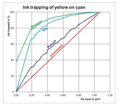
The graph ink layer versus trapping shows how differently the three calculation models see the truth.
