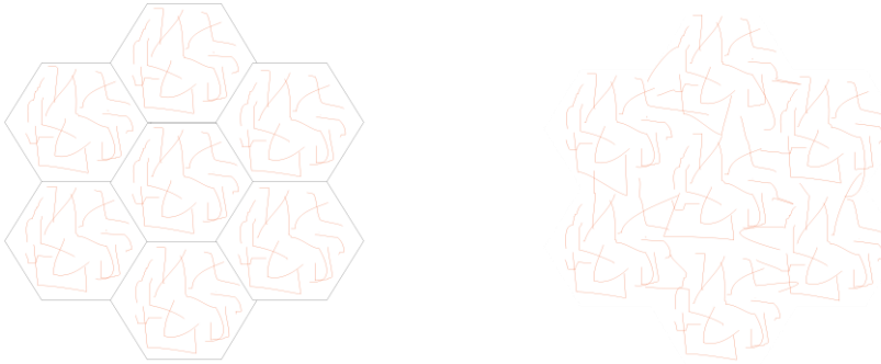
Fig. 13 Acrylate dispersions form films by interdiffusion. The interfaces between droplets vanish with the evaporation of the water
